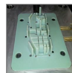
Core mold insert assembled to the mold base.
